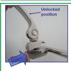
With the handle of the universal clamp in the unlocked position. Insert the lower jaw by pressure in the frame.
