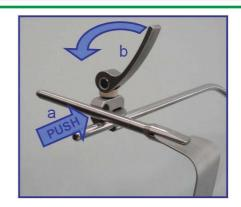
Insert the blade holder by pressure in the upper jaw of the universal clamp with the handle in unlocked position (a).
