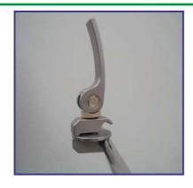
Despite the unlocked position of the handle, the universal clamp is held
